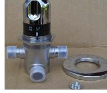
of of the cartridge spline to reveal the cartridge. For first fix protect the cartridge and valve body thrads from debris and damage by wrapping in an appropriate size plastic bage and securely taping in position with masking tape. The valve can be assemvle by following these steps in reverse and ENSURING the marks on the valve body thread, whitre vertical indicator line and oC are aligned when refitting.
