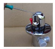
2 Using a small cross head screw driver undo the valve head retaining screw and safefly put to one side
