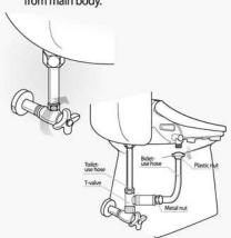
Press the button on the side of bidet, completely drain the water out of the of the main body. While keep on pressing the button, pull the main body forward, and then remove it from the toilet.
