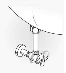
Be sure of no leakage around the hose connection.
